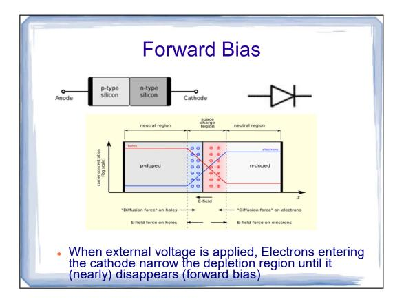
(have students draw a battery and attach to the diode to show forward bias. Draw the electrons and effect on the ions)
