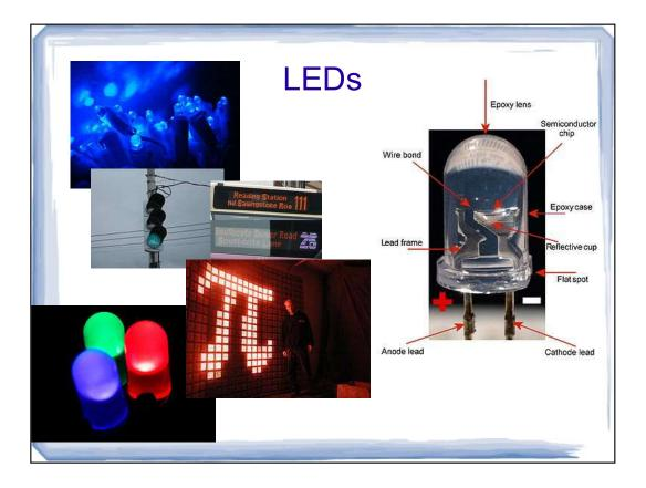
The P-N junction, when it is forward biased, not only conducts, but also emits photons (sometimes in the visible spectrum)
